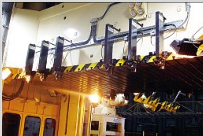
Alla Auto Clamps i parkeringsläge All Auto Clamps in park position Alle Auto Clamps in Parkposition
